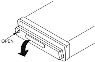
2. To remove the front panel, lift it up at a little angle from horizontal position, then first pull out the right side and then pull out the left side.
