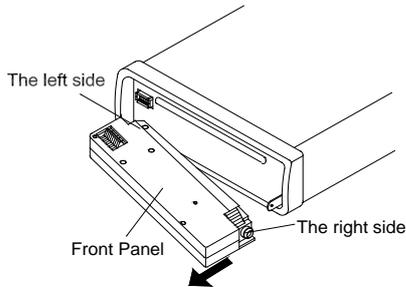
3. For safekeeping, store the front panel in the supplied protective case immediately after being removed.
