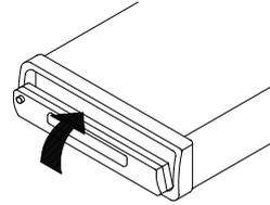
3. Note that if the front panel fails to lock in position properly, pressing control button may not function and the display may be missing some segments. Press the release button and then reinstall the front panel again.
