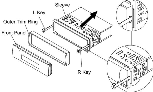
6. Mount the sleeve by inserting the sleeve into the opening of the dashboard and bend open the tabs located around the sleeve with a screwdriver. Not all tabs will be able to make contact, so examine which ones will be most effective. Bending open the appropriate tabs behind the dashboard to secure the sleeve in place.
